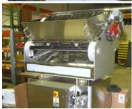
The SC-72 Slat Counter uses 42" slats to fill 12-20 bottles per index cycle.
